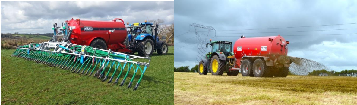
Figure 16: Example of modern low emission trailing shoe slurry spreading system (left) and traditional high emission ‘splash plate’ slurry spreading systems (right). (Images used by permission of Hi Spec Engineering Ltd. www.hispec.net )
